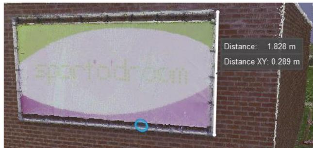
**Advanced Mode** displays all of the information that is currently presented to the user including the coordinates of each point plus the slope (linear) measurement and the horizontal (XY) measurement.
